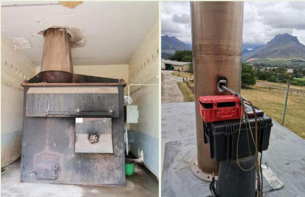
**Images 1 and 2:** In-stack monitoring for cremator's annual stack emission sampling
